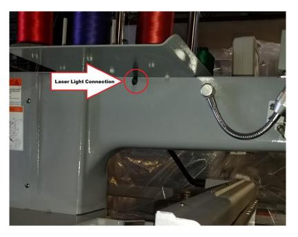
Simply connect the power cable for your laser to the connection site and mount it to the Side of the Arm of the machine. The Laser Assembly has a magnetic base so it will hold fast to any metal surface.
