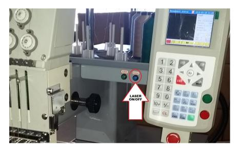
Once the laser is lit up; you will want to position the laser beam onto the needle plate hole by adjusting the angle of it. If you cannot see the laser light, use a white piece of paper to see where the laser is currently focusing it and adjust it so that the laser shines directly into the needle plates hole.
